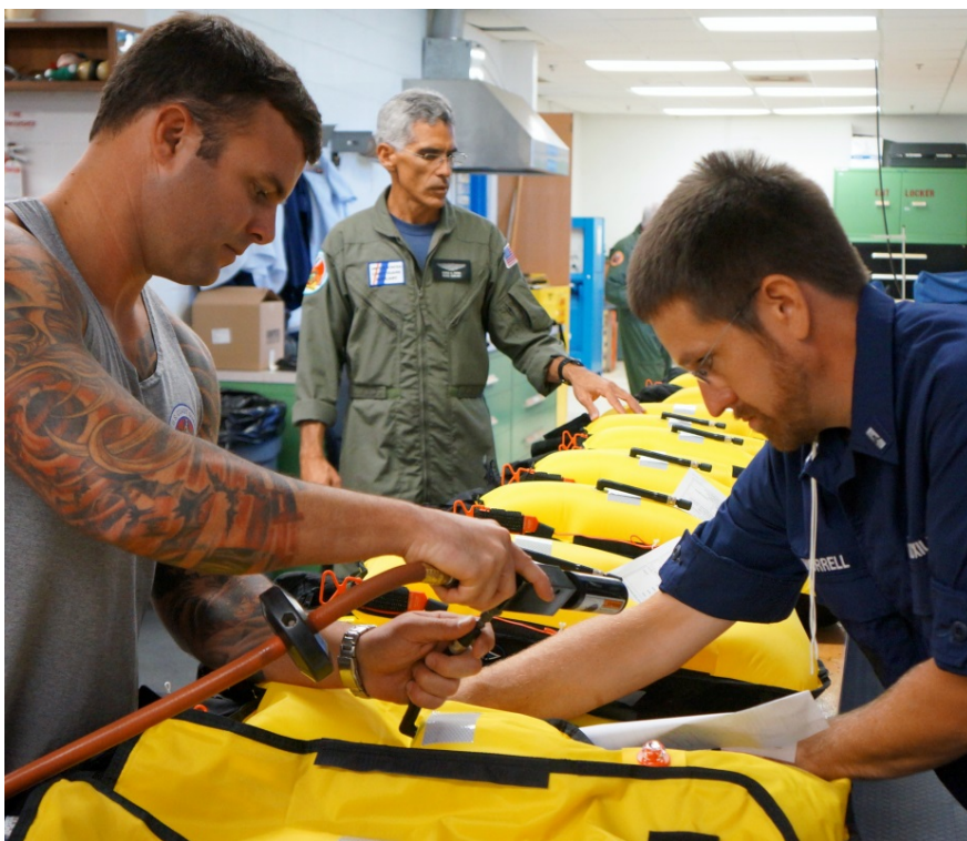
Auxiliary and Active Duty work to inspect and repack 30 Aviation survival vests in BQN's AST shop supporting AuxAir.
